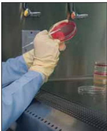
△ **Curved stainless steel air foil\*** gently supports the user's forearms without the need for a separate armrest. The radiused edge prevents the potentially dangerous practice of placing materials in this area. Contact Labconco at 800-821-5525 or 816-333-8811 for ordering information on an optional bold orange epoxy coating to caution operators to avoid storing or placing materials near the air foil.
