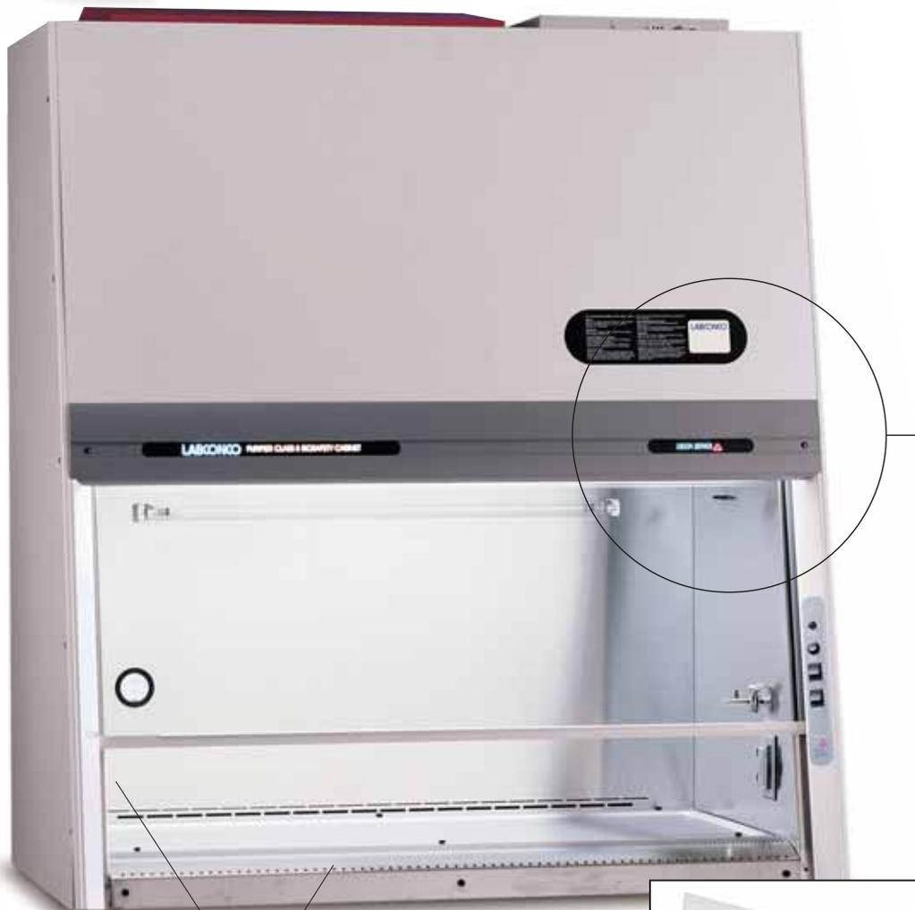
The patented \* Air-Wave™ Entry System, featuring aerodynamic angles surrounding the access opening, provides less airflow resistance for better containment.
