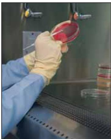
△ **Curved stainless steel air foil\*** gently supports the user's forearms without the need for a separate armrest. The radiused edge prevents the potentially dangerous practice of placing materials in this area. Contact Labconco at 800-821-5525 or 816-333-8811 for ordering information on an optional bold orange epoxy coating to caution operators to avoid storing or placing materials near the air foil.
