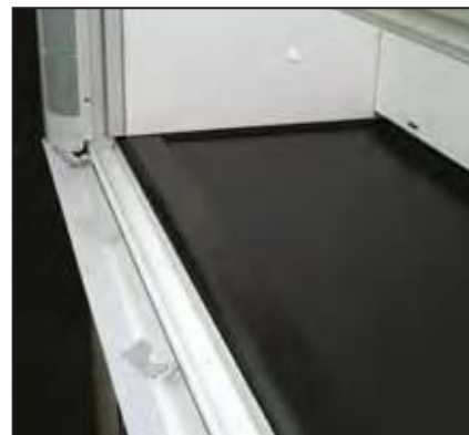
The integral spill trough prevents spills on the work surface from leaking out the front of the hood. The air foil pivots up to provide access to the spill trough for cleaning.
