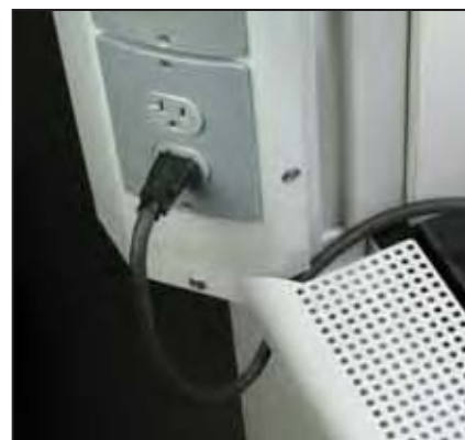
Openings on both ends of the air foil allow electrical cord pass through without disrupting airflow. Cords do not block airflow and are out of the way of the operator.
