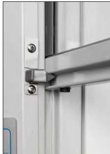
The sash latch holds the sash in the 28" high position for loading. When the latch is released, the sash automatically returns to the 18" operating height position.
